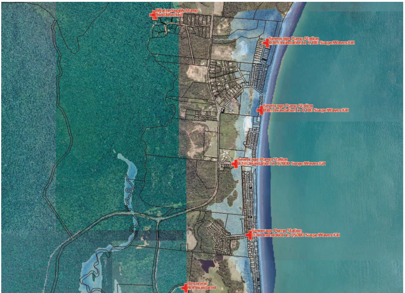
Figure 5-11 Inundation of Critical Infrastructure: Wongaling Beach
