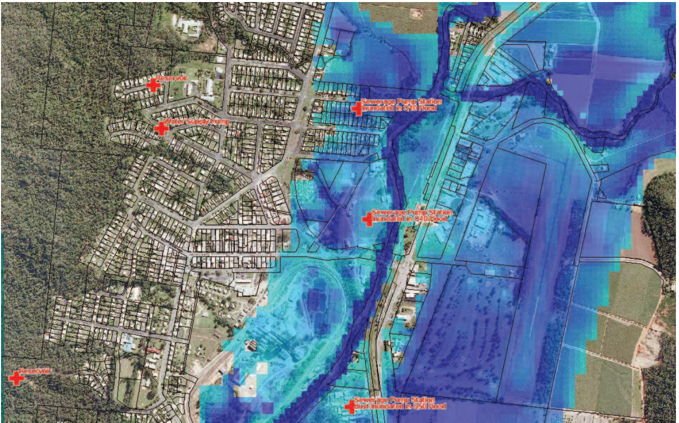
Figure 5-9 Inundation of Critical Infrastructure: Tully
