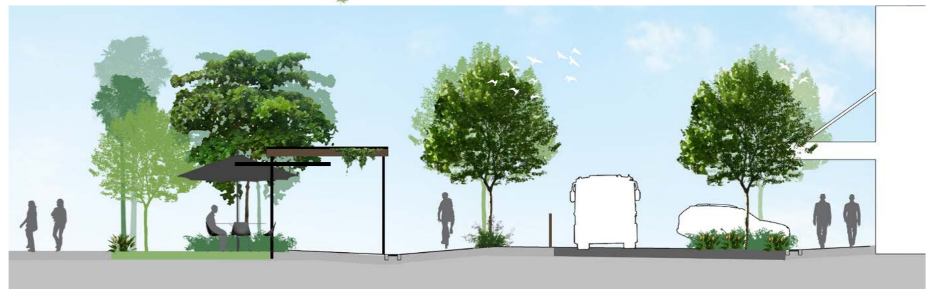
Footpath & Turf Breakout | Pedestrian Plaza & Arbor | Traffic Lane | 4.8m 45° Car Parking | Footpath Typical Cane Cutter Court Cross Section
